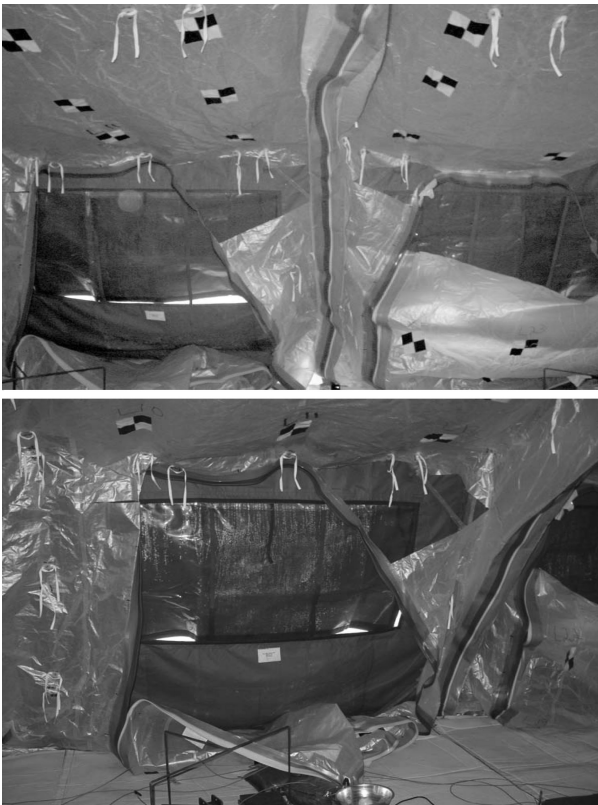
Fig. 2 Blast damage to TEMPER tent liner on back side.
